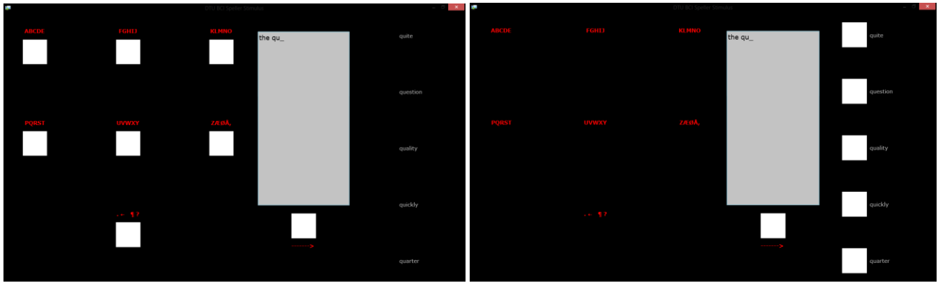
Figure 2. DTU BCI Speller interface. The left figure shows the interface when a user is selecting characters. The right figure shows the interface when a user is selecting a dictionary word.
